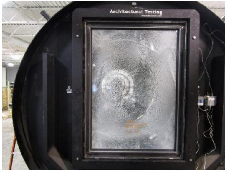
Photo No. 8 Post-test Specimen #3, Interior
