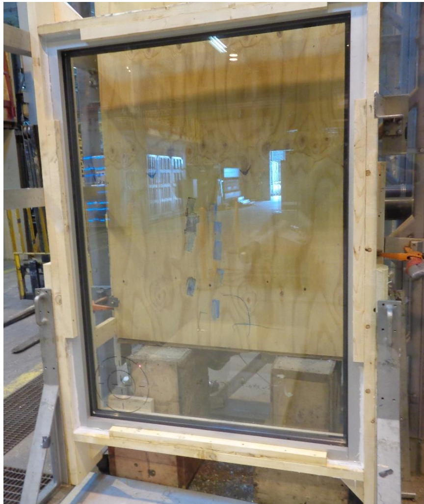
Photo No. 1 Test Specimen After Air, Water, and Structural Testing
