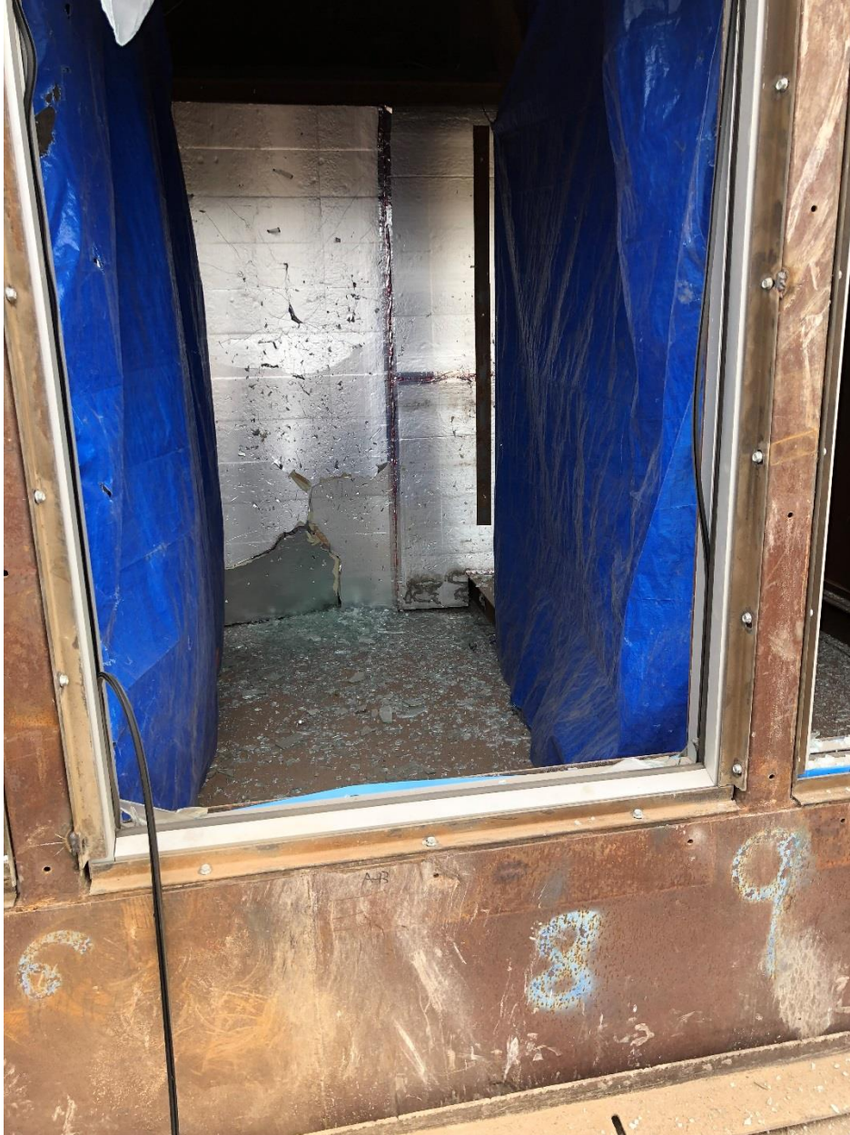
Photo No. 12 Post-test Specimen Annealed No Film exterior
